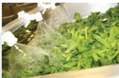
One of the 5 washing steps in the IV range production plant in Manerbio
